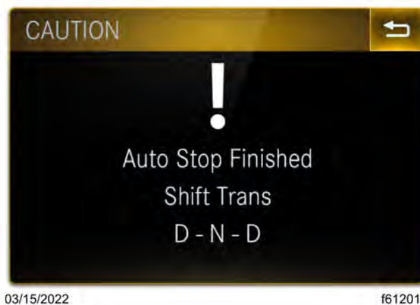
Fig 148, Auto Stop Finished Caution, ICC5
