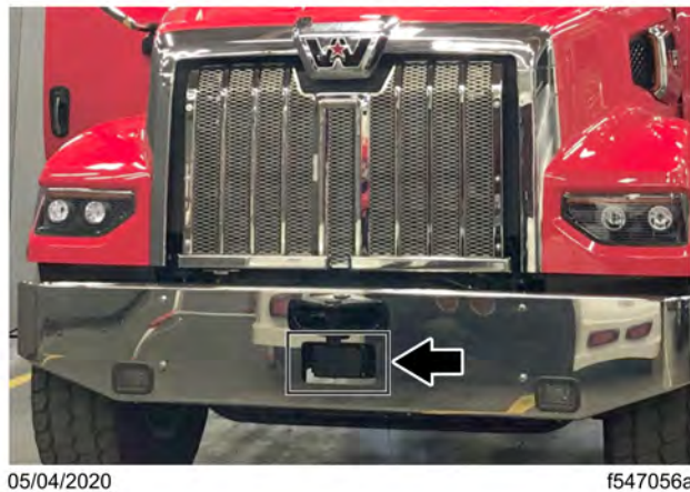
Fig 131, Forward Radar Location
