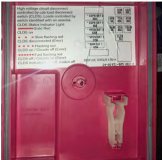
Fig 242, Example Fuse Labeling on BCA Cover
