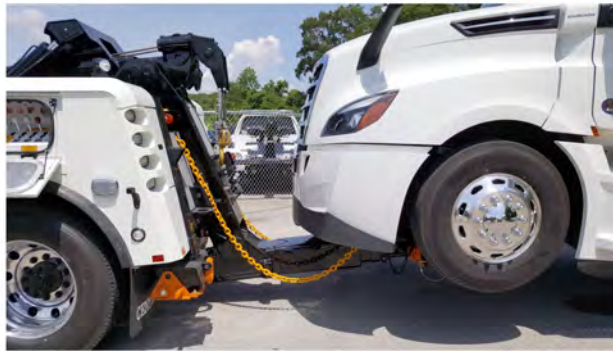
Fig 385, Safety Chains Connected on the Towed Vehicle
