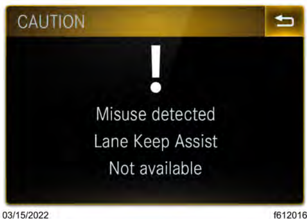
Fig 149, Caution that LKA is Unavailable Due to Detected Misuse - ICC5
