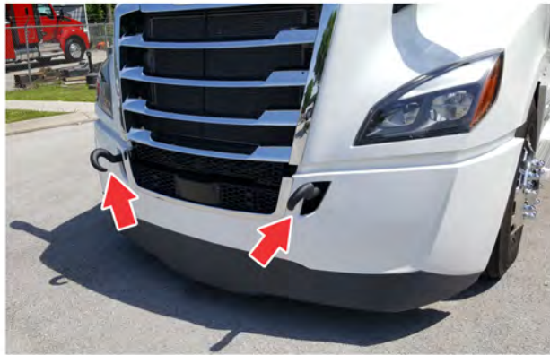
Fig 375, Tow Hooks Installed, Facing Down
