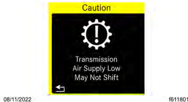
Fig 293, Low Transmission Air Pressure Pop-up
