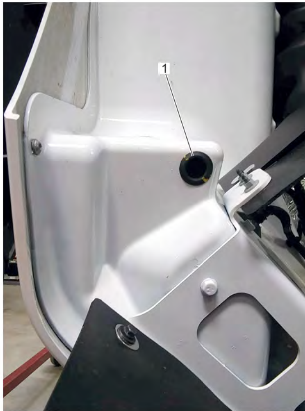
Fig 354, Headlight Adjusting Opening (shown with hood open)
