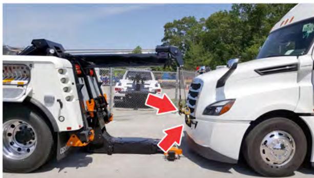
Fig 377, Tow Cables Connected to the Tow Hooks
