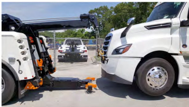
Fig 378, Moving the Stinger and Crossbar Under the Bumper
