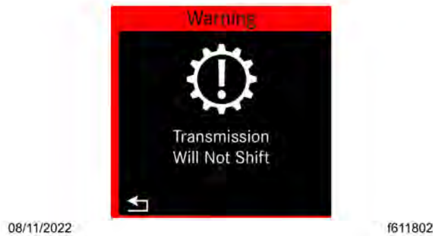
Fig 297, No Transmission Air Pressure Pop-up
